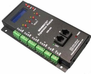
The SoundStik Expansion Module is used with one or two SoundStik-mp3 handsets and 0-4 remote push buttons. The system can store, play and track usage for 1 to 4 mp3 files.
