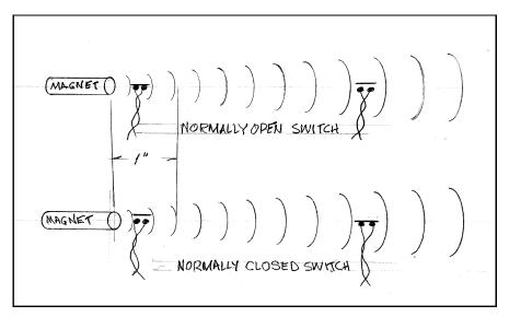
SoundStik internal switch prevents or allows current flow when within about 1" of Hanger Mount magnet.
